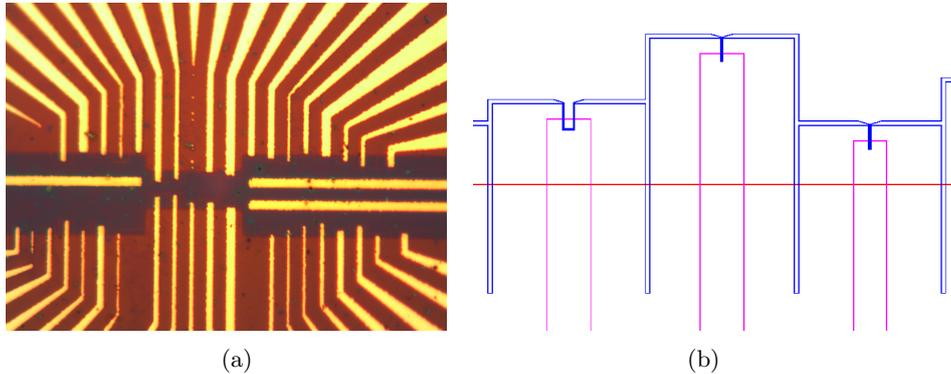
Figure 10: Left: picture I took of a finished device prior to measurement. It can be seen that the finger the middle top finger did not develop properly on this device. This is due to errors in optical lithography. Right: AutoCAD design of fingers on graphene developed using EBM
