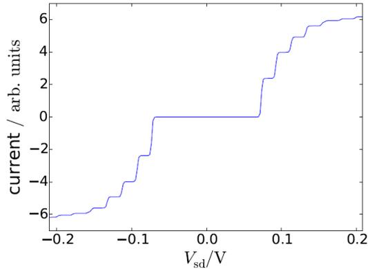
Figure 4: Idealised example of Coulomb staircase I-V diagram
