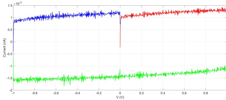
Figure 13: Open contact I measured on the device EBD50A. Data plotted in red and blue was from ramping the voltage up, while the green one was from ramping down. Noise and offset of about 1.2pA due to capacitance of wires are visible.
