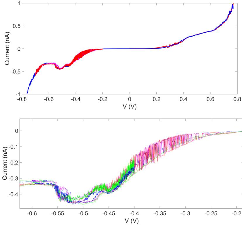
Figure 17: An example of a reproducible NDR I measured. Full curve on the top and zoomed in NDR over many runs on the bottom. It can be seen that the curve has additional step like features and switching of channels around the NDR implying possible nanocrystal charging and a transition to a different stable state.
