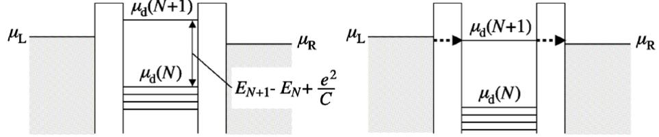
Figure 2: Coulomb blockade in a quantum dot: (a)no energy levels between source and lead electrochemical potentials, tunnelling suppressed (b)electrochemical potential of the  $(N + 1)^{th}$  state between source and lead electrochemical potentials, tunnelling possible. Picture from PNS course [4]
