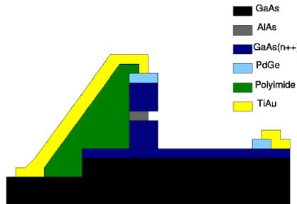
Figure 6: Device cross-section after processing and etching of the AlAs layer. Picture from Ref. [13]
