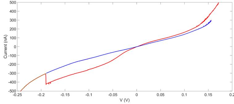
Figure 12: Contact on device EBD40E which displayed change of behaviour. Initially, the behaviour would follow the blue line, but when higher currents were tried, the behaviour abruptly changed to the red line
