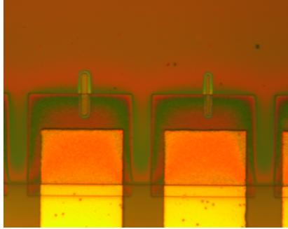
Figure 7: Microscope picture I took displaying pillars with exposed windows. For size reference, thickness of the gold fingers is  $80\mu\text{m}^2$
