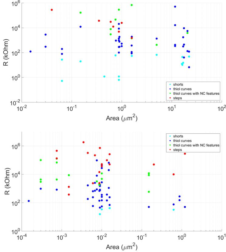
Figure 18: Log-Log plots of average resistance against the nominal area of junctions for different types of curves in devices with diluted NCs samples (top) and pure PbS NCs samples (bottom).
