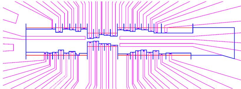
Figure 9: AutoCAD mask design used for optical lithography, realised by J.M. Fruhman. Purple: gold fingers. Red: graphene sheet. Blue: EBM lithography
