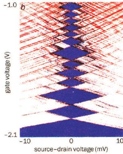
Figure 3: Grey-scale plot of the conductance of quantum dot dependant on gate voltage and source/drain voltage. Lighter regions imply higher conductance. Picture from PNS course [4]
