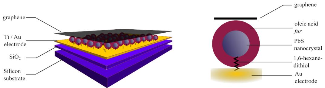
Figure 8: Structure of the device. Left: layered structure of the device. Right: electrically contacting nanocrystal cross section. Picture taken from Ref. [1]
