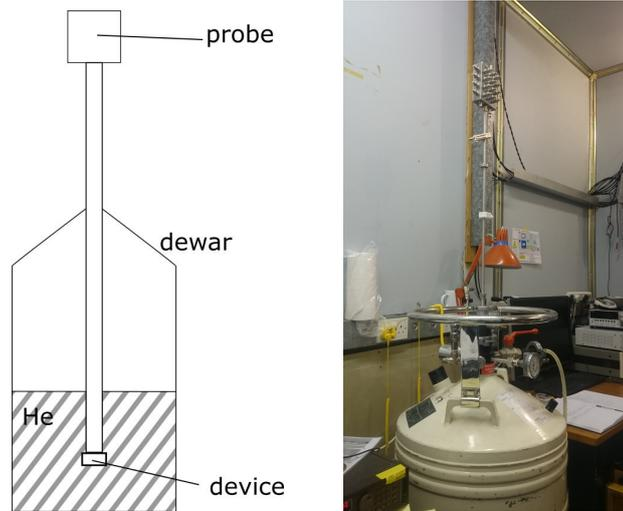
Figure 11: Sketch and a picture of the dewar I used for the measurements
